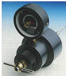
Load Test Unit
