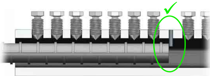
Figure 1. Correct Rebar Insertion Depth
