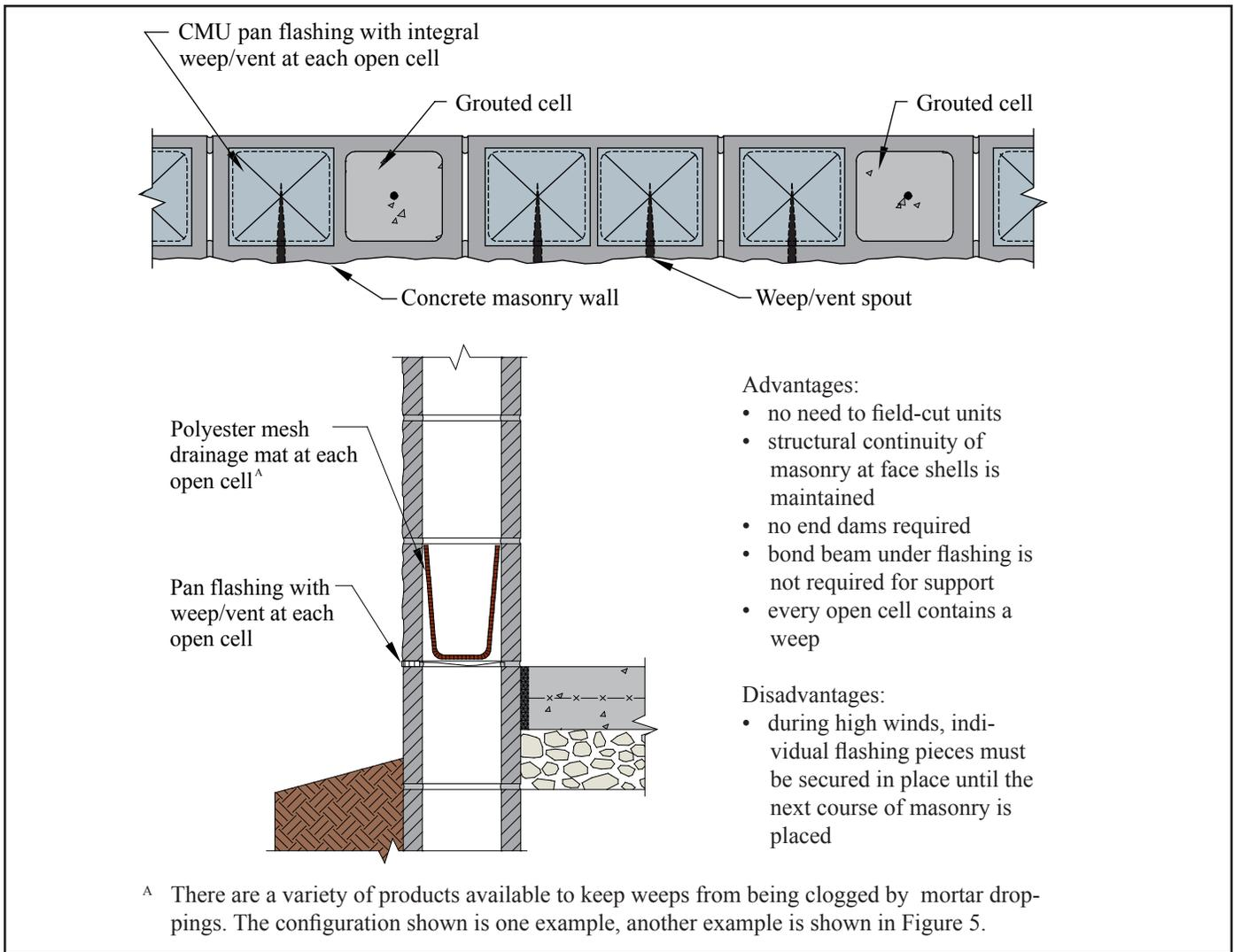
**Figure 4—Pan Flashing with Integral Weeps**
