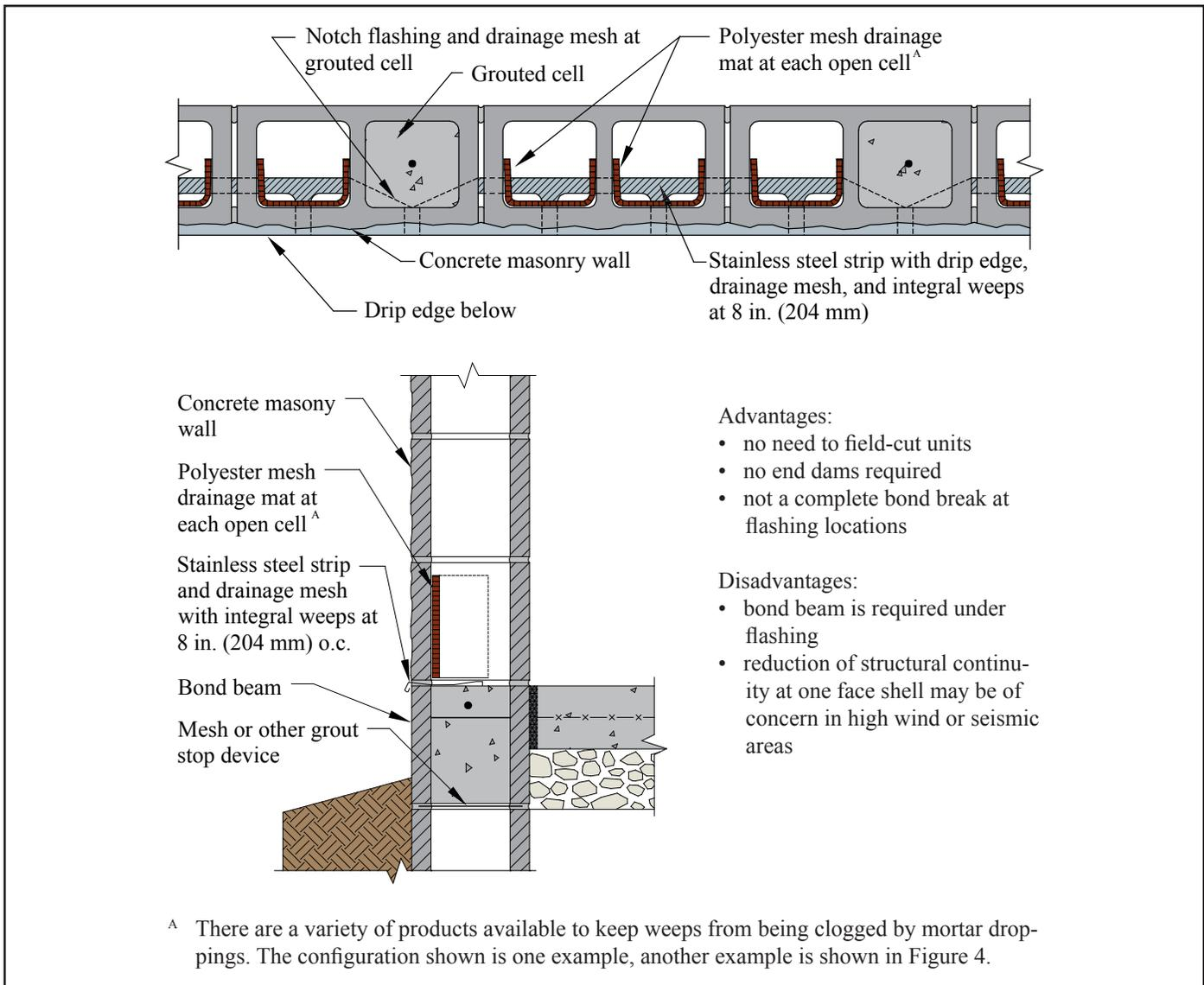
**Figure 5—Stainless Steel Strip with Integral Weeps**
