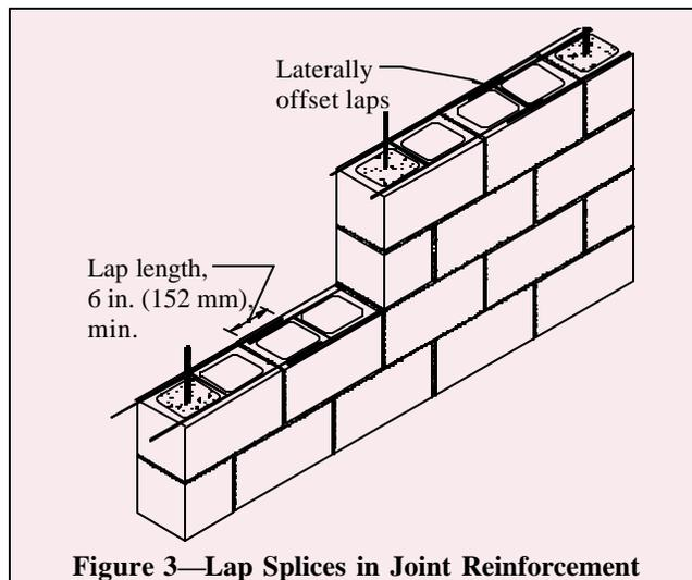
Figure 3—Lap Splices in Joint Reinforcement
