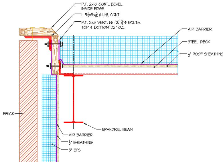
**Figure 4:** Wood support for roof edge angle.
