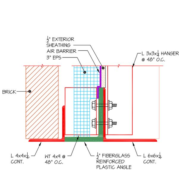
**Figure 2:** FRP angle used as shim in hung lintel for thermal break.
