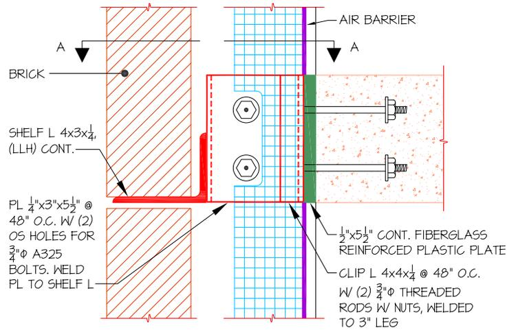
**Figure 1:** FRP plate used as shim and edge form at relieving angle for thermal break.
