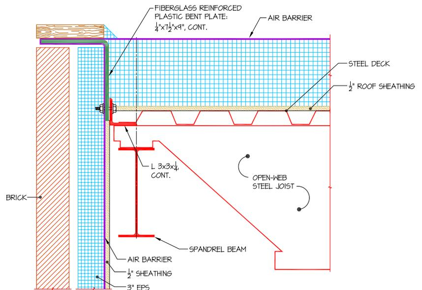
**Figure 3:** FRP angle used for roof edge angle support.
