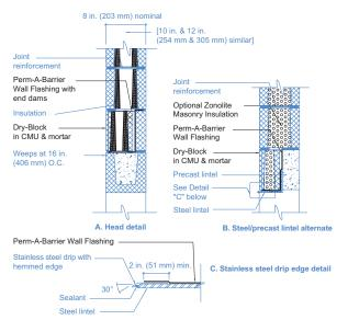
**Masonry Opening Head Flashing**
