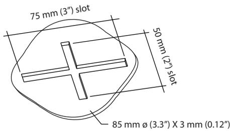
Figure 2 Insulation Support/Retainer
