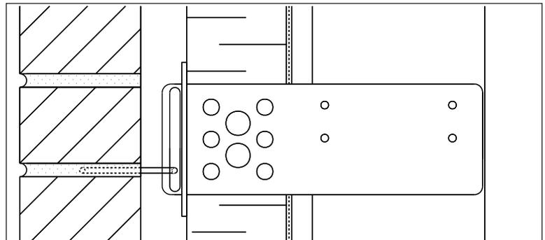
Figure 5 Slotted Stud Tie (Type 1) Installed
