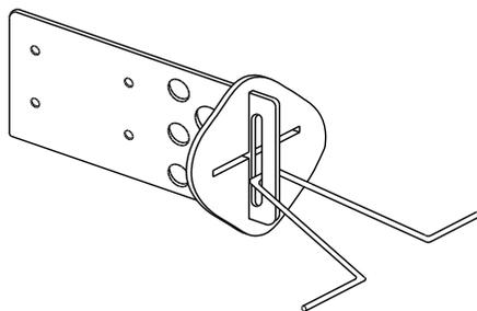
Figure 4 Slotted Stud Tie (Type I) Assembled
