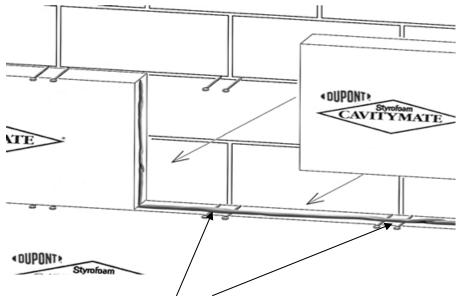
Continue the PL300 over the adjust. ties to adhere the insulation to the substrate.
