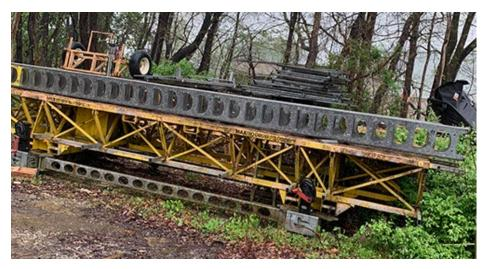
(3) - Alimak electric mast climbers. 60'x 80'. Ready to use. \$18000 each. 12000# in 60' setup, 7500#s of capacity 20 to 30' per min travel.
