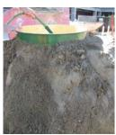
Step 3. Insert the Volcano Rod into the drum then plug it in to 120-volt grounded outlet with GFI (ground fault interrupter). Do not energize the unit unless it is
