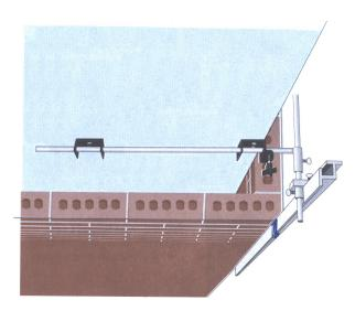
The **Post Speed Lead** needs only one bracket after the first brick is laid. The bottom of the vertical pole is held against the brick by the tension of the line.
